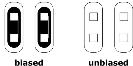
*Network biasing is applied with biasing jumpers*
