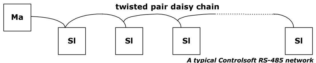
All devices on the network receive any transmitted data. The device for which the data is intended responds if necessary.
