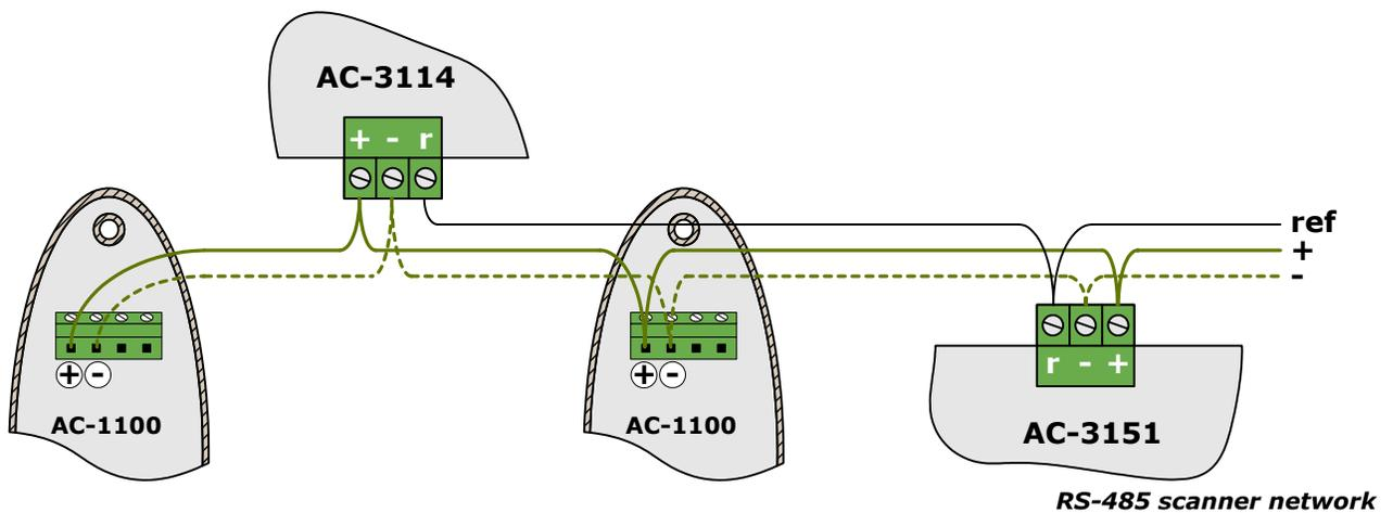
The diagram above shows a standalone RS-485 network. The AC-3114 controller can host up to 16 slave devices.
