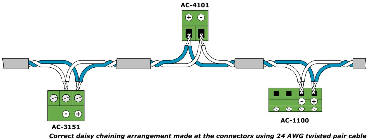
The finished network should have all + connection points linked to the + line and all - connector pins linked to the - line. The network lines are distinguished by the conductor insulation coloring or marking. The diagram above shows the + line in blue and the - line in white, though the actual cable coloring will vary.
