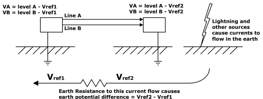
The RS-485 standard accommodates an earth potential difference of up to 7 volts. Therefore, if the difference in the earth potential between two points of signal interpretation is greater than 7 volts, the data may not be correctly interpreted from the signal levels. Furthermore, the earth potential difference may damage the network drivers.
